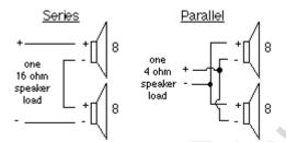
For series connections, always connect the (+) terminal on one speaker to the (-) terminal of the next speaker. For parallel connections, always connect (+) terminals together, and (-) terminals together. This keeps the speakers all moving together, delivering the maximum amount of sound possible.
