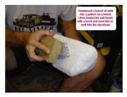
Press the hot nails into the styrofoam about an inch. You have to be very careful and go straight in and pull it straight out.
