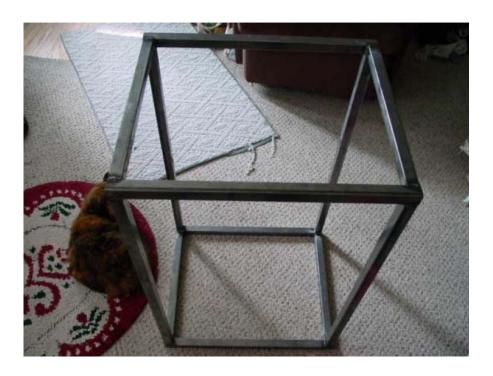
Next, risers are welded at the corners of one of the sections. Again, welding magnets make this easier. When that's finished, the other section is placed onto the risers, indexed properly into place with magnets, and welded to form a basic enclosure.
