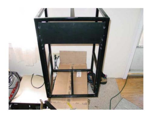
If all goes well, faceplate filler panels, shelves, etc. should drop right in without interference or alignment problems.
