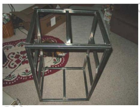
The next step is to weld in the remaining 16" pieces that will serve as supports to reinforce the frame. One per side is centered into the top and bottom, and two into each side. These help distribute weight from the rack rails and help prevent the tubing buckling under extreme loads.
