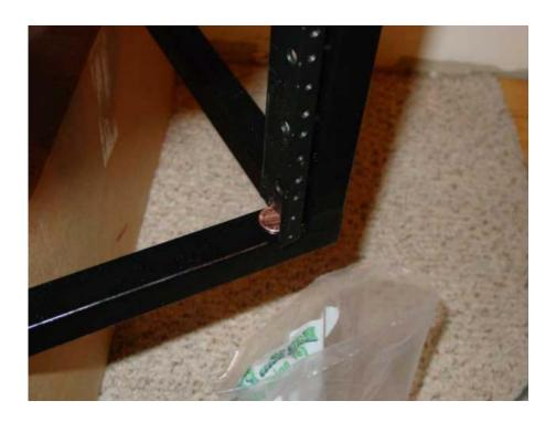
With the frame finished, the rack rails can be mounted. Since the design leaves the rack slightly larger than required, the rails can be centered into the frame vertically by using something to gap the bottom of each rail up from the bottom tubing. A cheap but workable tool for this is an ordinary coin of roughly 1/16" thickness, such as a penny.
