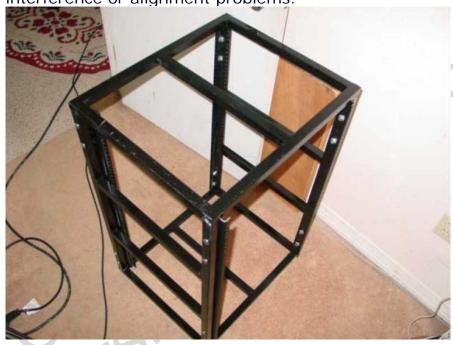
At this point, the rack cabinet frame is complete enough to use as-is, or you can attach side panels to the frame using whatever hardware you need. One nice-looking (if a bit pricey) suggestion is to drill and tap holes and use cap screws to attach the side panels, and use tinted acrylic for the side panels themselves.
