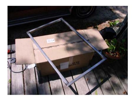
Once the cut work is done, two of the 31 3/4" lengths and two of the 21 3/8" lengths are welded to form a rectangle. This is repeated to form the second. These will be the front and back openings and rack rail support struts for the rack cabinet's frame. Welding magnets make this process easy, by holding the tubing in place and keeping the angle 90 degrees.
