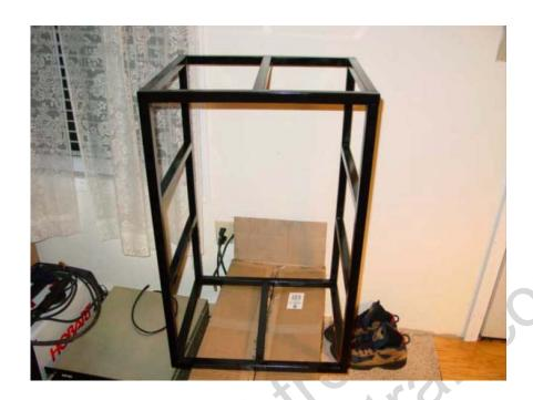
The next steps are to clean the frame thoroughly, and then to paint the frame completely with primer and then a good quality paint. This isn't intended to be cosmetic so much as to prevent corrosion – exposed steel will eventually rust.
