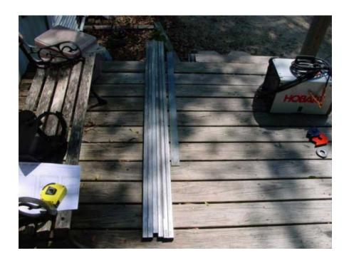
The material chosen was 0.62" wall, 1" x 1" square steel tubing. This tubing is widely available at home-improvement stores and usually costs about \$7 for a 6-foot length. For this project, six pieces of 6-foot tubing are required. As an option, a flat metal bar can be used to create corner reinforcements that double as mounting points for casters.
