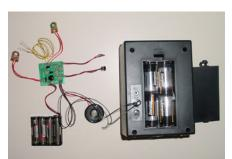
Congratulations! At this point you've made all the wiring additions needed to form a portable haunt sound system which may be triggered, in addition to the manual "play" button, by an external switch connected to the two yellow wires.
