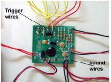
The other ends of the two wires from the mini-plug are soldered to the existing "solder mounds" of the two speaker wires. There is no polarity. That means: it doesn't matter which wire of the two goes to which solder mound. In the above photo the two black wires from the mini-plug are shown soldered to the same mounds as the two red wires from speaker.
