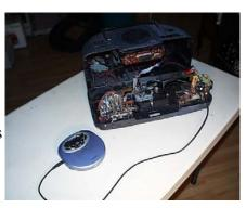
With the two units now connected with your test patch cord, turn on your audio source and press play. This test proved successful in using the cable that went to the amplifier from the radio. In the next picture we will show you how to use the other sources of your boombox if a radio isn't present or just unavailable.
