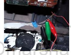
Here is a picture of how I probed wires into the CD player cable of the same boom box. The resistor you see here is merely being used as a piece of wire to reach inside the ribbon connector and has nothing to do with accessing the amplifier.
