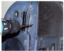
You've done it!! Now all that is left to do is make the connections permanent. One way to do this is to drill a hole in the case of the boom box and run your audio test cable through and solder directly to your predetermined connections. After soldering the wires, they must be individually insulated by either wrapping them in electrical tape or heat shrink tubing. The cable is now ready to plug into your external audio source.
