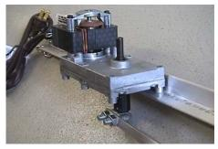
In this shot you can see we have attached the motor to the motor mount angle portion of the platform on one side of the motor only. Don't be worried that you need to support the motor on the other side, as the angle mount is more than strong enough to keep this from flex of any kind during use.
