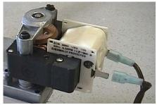
Next, chop the female end off of your power cord and crimp insulated 1/4" female terminal disconnects to each lead and plug into the two male fittings on the back of the motor. Use 2 zip ties to secure the power cord to the side of the platform as seen here.
