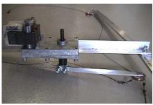
At each end of the arms and at the back of the motor platform you will need to attach your S hooks. One to attach your cord to which will suspend it from the ceiling, the other to attach our pulley.
