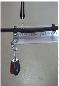
Here you can see that we have another S hook in the top hole, just barely above the power cord for suspending the back portion.
