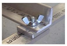
Now is a good time to attach the two platform arms. Place the 1/4" bolt through the ends of both arms and then the platform, tightening down with the wing nut.
