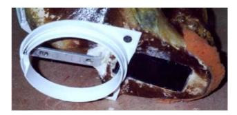
The hollow core of the skull I chose allowed for me to fabricate and install a mount made out of flat aluminum stock that was 1/8" thick, 5/8" wide and about 14" long.
