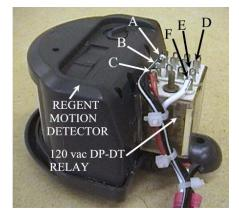
While this little goodie shown here was not used on this particular how-to showing how to set up a fully automated sound and trigger system, I wanted to add this section here so you could see how you can solder up your own relay in a very small, compact package that has the capacity to totally isolate trigger signals.
