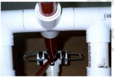
The funny looking blue thing in this photo is a washing machine water solenoid that we will be using for our <u>Air Trigger</u>. The needle valves (shown in the pic at top)(2) should be a standard 1/4" valve from the local OSH or other hardware store, (Anderson Barrows Tubing to Tubing Straight Needle Valve Part No#BP9106-CP 1/4"). You will also need 20' of 3/8" rubber airline and 1' of 1/4" plastic tube for attaching to the needle valves, shown attached to the valve at the top right.
