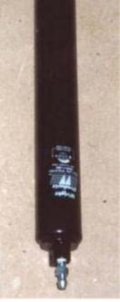
cylinder cylinder . Now you will tap threads for the automotive bleeder screw but stopping just shy of the end of the hole just as you did with the drill bit. You will notice the bleeder fitting has a hole running down the center of it that then stops at a junction that routes the brake fluid to each side of the screw.
