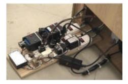
Shown is a 120V, 4 Pole, Double Throw, KH style or "Ice Cube" relay. Nicknamed that since these relays are always covered with clear shells so you can actually see inside. That must be for geeks like me that have to see it before I can understand it. I work with these as they are readily available from surplus places such as All Electronics for just a few bucks. Ice cube relays come in different volts and amps, so be certain about your needs before choosing the one you will work with.
