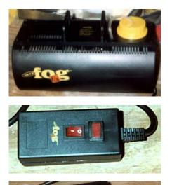
So using the fog machine as an example of just how this works, you should get a pretty good idea how to use this for the other items which are triggered by passively connecting a single circuit. In this photo you can see the wired hand held remote control with a switch in the middle. Since I need so many items to go off at the same time with this prop it isn't practical to try to do it by hand, hence the reason for the conversion.
