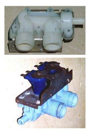
Of course you will need a water valve from a washing machine and not just any valve will hold the air back and reseat itself under the rather high pressure I would need for an air cannon. I wound up testing many, many different valves to see which work and which don't. There are two that I have had success with at high pressure such as what my <u>Aerial Executioner</u> operates at, some 85 lbs.
