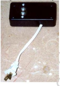
I just cut a slot out of one side of the box, drilled two holes and mounted the attachment board facing out. I also had to grove a hole out from between both top and bottom sections to get the power cord out. Now we are ready to put this to use.
