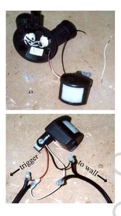
First thing is to disconnect the detector from the rest of the assembly as shown here. There is an extra length of wire that is used in the attachment to the light sockets that you will want to save for the next step. On close inspection of the photo you can just make out two wire couplers on the lower left. One is for coupling two small electrical wires and the other is one size larger that accepts three wires.
