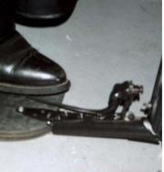
The other end of the short 5" to 6" section is attached to the wood platform with another hinge. Notice that this hinge is only attached to the board with one screw and even that one is not tight. This attachment is loose on purpose.
