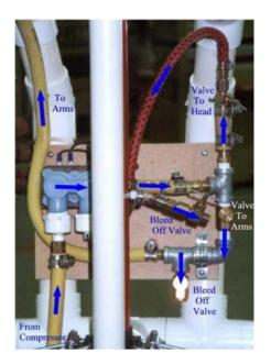
You should be able to duplicate the assembly above using the materials list from the previous pages. The 3/8" air line is clamped to the trigger output, then to a slip airline fitting that is threaded into a T that will go off to both the head and arms. For the line going to the arms the air then goes through a all thread fitting, into a trim valve and into a 90 degree elbow to another all thread fitting and into another T.
