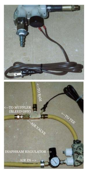
And here is how it will look when completed. The top of this photo got cut off, but you can see that 3/8" air hose slips perfectly over the outlet nipple for feeding the air to your prop. And that's it!
