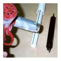
We need to install the forearm air rams at this time. First you will slip your 3/8" rubber air line over the end of the brake bleeder and then push it up over the hex teeth you use to tighten the fitting with.
