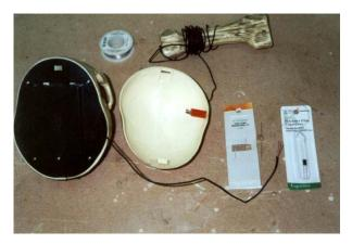
After a great deal of help from the folks on the <u>chat</u> <u>list</u> I was able to find a capacitor and resistor that would allow me to use the headphone out jack on my cassette player to send a signal to the line that the microphone attaches to on the Boris. Radio Shack carries this .01pF Polyester Film Capacitor and the 10K ohm resistor you will need. The photo above shows a picture of a 470 k ohm resistor, but it turned out that the correct one is the 10k, so substitute the 10 instead.
