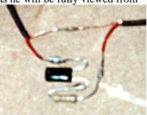
the center. It is of note to mention here that this took days to determine the exact capacitor / resistor combination that will make this work at a level that is audible by using the headphones out jack of a cassette player. However, this will not work with a little handheld player or little CD player as they simply do not deliver enough volume. You must use one of the larger players meant to be listened to like a stereo in your room.
