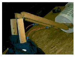
Using the strap hinges, attach the lower legs to the upper legs placing the hinges on the reverse side as the 'T' hinges (knee joints).
