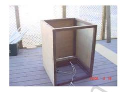
Next we built a drop-in wall behind the front wall that will channel the air up the inside front of the well. I left a gap in the middle of the inner wall (partly on purpose to route fog into the channel as well; partly because I used two scraps of wood I had leftover for the channel and they didn't cover the entire width.)
