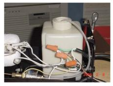
Basically I just identified the wires that fed each side of the switch on the remote, traced them back into the unit, and added my own leads to the wire-nut bound connections. I drilled a small hole out the back of the unit to feed my new wire, and ran that wire to the K1 blocks on the RC-8 board. Here's a close-up of the innards of the fog machine with my new leads attached;
