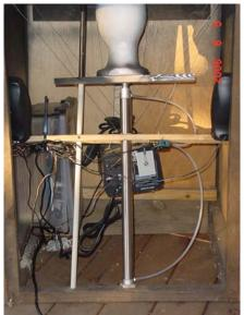
You can also see the 1x4 mounted onto the top of the cylinder, to which I attached the foam head (wire wrapped over it and secured to staples under the board; a strip of duct tape under and on top of the wire protects the foam head). Also note the thin PVC tube I mounted to the left of the cylinder; it is secured at the bottom and provides a "guide" so when the head/platform raises and lowers, it won't twist or turn to either side.
