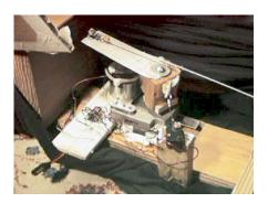
The metal lever rotates freely on the wooden base which is attached to the motor. As the base rotates, a screw sticking up from the base catches the lever and pulls it around raising the Flailer's arm. The motor is stopped just short of pushing the lever all the way around. To release the arm, the motor simply starts running again and pushes the lever past the critical point. Then the lever is pulled around, away from the screw, by the arm's elbow springs.
