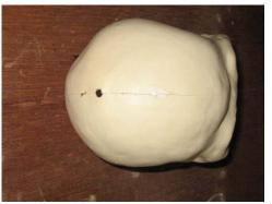
This hole is needed to attach the servo to the horn and can easily be patched over later.
