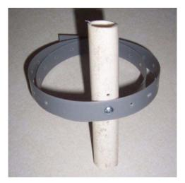
Step 3 - Secure the plumbers tape to the PVC pipes using a 6x1/2" sheet metal screw. This was secured at 8" from one end of the tape.
