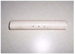
Step 1 - First, drill some pilot holes for the tape to be secured to. I found that this step makes the movement adjustments easier later in the assembly
