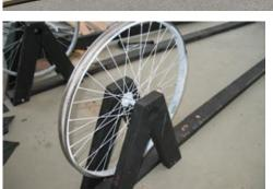
The joints fit together perfectly to form the complete circle. Note that I'm now using "T" nuts instead of loose nuts as shown in the above picture.
