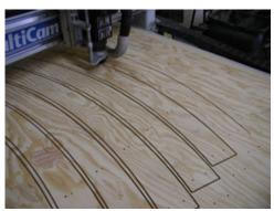
The individual pieces are cut from 1/2" plywood using a CNC router (thanks Jim). The accuracy of this device is absolutely amazing. If you're interested in getting your own set of hoops made, you can <u>contact Jim</u>. I think he charges about \$250-\$300 plus shipping for a set of three hoops.
