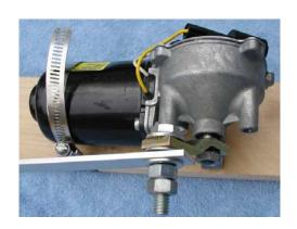
You need to attach the aluminum bar to the motor. Using the 5/16" bolt, three washers and two nuts, assemble as shown left, through the 5/16" hole in the bar.
