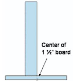
Next, we'll join the two boards together. Line them up as shown at left, with right side of the 3" board aligned with the center line of the 1 1/2" board (this will place the drive side of the motor below the center of the chair).
