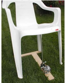
This is a picture of the mechanism we'll be making. It consists of a plastic chair, a "T" shaped piece of wood, a wiper motor and an aluminum bar to connect the motor to the chair. It should cost less than \$35 for everything.
