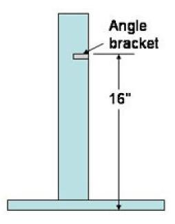
In this step, we'll install the angle bracket that will be used to mount the motor. Mark a line on the 3" wide board about 16" from the back edge of the 1 1/2" board (this distance may vary depending on the chair).
