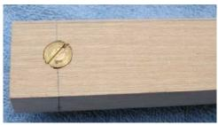
Drill a hole in each end of the 1 1/2" wide board to match the holes in the chair legs. This hole needs to be big enough to accommodate the "T" nut, which should be about 5/16" diameter.
