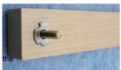
Countersink the hole so the 1/4" screw will fit flush with the bottom of the wood. Insert the "T" nut into the top side of the wood and then screw in the screw.
