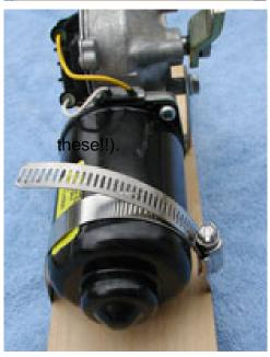
We need to remove the ball from the arm that's attached to the motor
