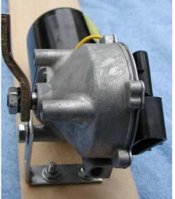
To mount the motor, you'll need to enlarge the top hole in the angle bracket to accommodate the 6mm screw for mounting the motor. Use a 1/4" drill bit (or 6mm) to drill out this hole.
