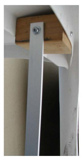
My chair did not have these ribs so I had to add a 2x4 block of wood as shown left for the mount. You'll have to adapt your chair as necessary. I used a 1" #8 wood screw and washer to mount the bar to the block of wood.
