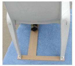
To complete the project, place the chair legs over the screws on the rear board and then install the 1/4" lock nuts. Tighten the lock nut just enough to engage the locking material but be sure to leave a gap as shown right to allow the chair to rock freely. The nut is just to make sure the chair does not come off the screws.
