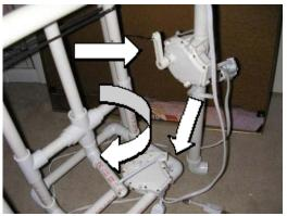
Here you can see the motor placement and the arrow is pointing to the "swing" point. The 1/2" PVC just sits loosely into a 3/4" tee. This allows the center portion (seen better above) to swing free as the motor moves it.
