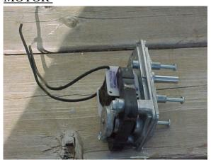
We used a Dayton 4RPM AC Gearmotor, item 3M098, that my husband picked up at Grainger for \$34 (<u>click here</u> for instructions using a rotiserrie motor). We mounted it on its side to a small sheet of wood and then attached a block of wood to this as a base. This base we screwed into the bottom of the tombstone box. This keeps the motor stable and secure. Make sure you don't screw the motor to the wood sheet too tight or the motor will bind up and not spin.
