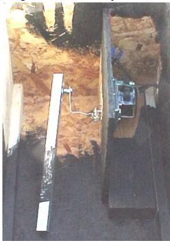
Here's how it looks with the motor mounted in place and the crank finished. The free end of the aluminum stock will be sitting in a PVC elbow that's screwed into the lid and this will make the lid rise and fall. We drilled a hole in the back of the box for the motor cord. We placed it a little higher than the motor in case of rain so the water wouldn't run down the cord and ruin the motor. For added protection we put a roof over the motor (not shown).
