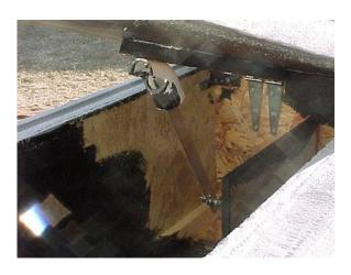
A view of how the crank works. The elbow PVC is mainly used as a device to hold the aluminum stock up. The stock isn't glued or screwed in - it's just set inside the PVC pipe. When plugged in the motor turns the shaft which rotates the L bracket. The aluminum stock rises and falls. The stock, which is Nestled inside the elbow pipe that is attached to the lid, lifts and lowers the lid.
