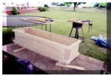
The main body of the coffin is basically...a box. The key here is to build this out of one sheet of wood. it measures 71" long x 23" wide x 18" tall (roughly 6'X2' and 1.5' tall).
