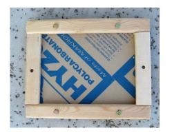
To make the window, I got a piece of plexiglass from a scrap pile at work. I, by the way, have no idea how to actually buy a piece of plexiglass so you are on your own. I then made a wooden frame and drilled holes through the frame and plexiglass.
