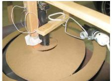
I then put a section of an empty cardboard role over the light and covered the end of it with toilet paper. This is to diffuse the light. I mounted the white light over the small wedges and the black light over the larger wedges.
