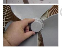
3.) The fan blade cap is unscrewed and removed.
