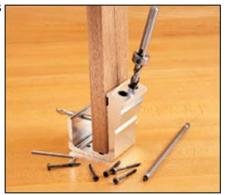
The jig shown here is a Pock'it Jig Kit you can order from a tool supply like <u>Woodcraft</u>. When making fine finish products with a jig such as this, you also need the special drill bit as well, so your center hole and counter sink are correct. For our project you can just wing it with a #8 drill
