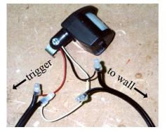
Now we will connect our leads to the detector. I use about 15' of cord going out to the trigger and about 5' going back to the wall socket. You can use standard zip cord and add your own ends to this arrangement, or you can simply purchase one 20' extension cord and cut it 5' from the male end and be done with it. Not
