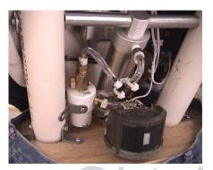
It turned out the air cylinder we used was double acting, which means it will push or pull the plunger.
