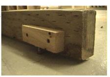
You will need a 3/8" drill bit to drill your hole under this block to tap in the threaded insert for this glide to screw in to. Then attach with a little glue and a couple of screws. Now you can instantly spin one or the other down to take up the slack from uneven concrete to keep this much more stable and from rocking while in use.
