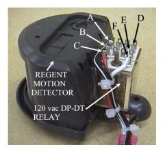
While this little goodie shown here was not used on this particular how-to showing how to set up a fully automated sound and trigger system, I wanted to add this section here so you could see how you can solder up your own relay in a very small, compact package that has the capacity to totally isolate trigger signals.
