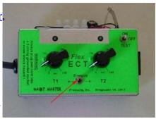
off and then keep it from being able to be triggered again for, say, 20 seconds. If you run two wires from your solenoid, or Interface, to the side attachments on this ECT it will detect the circuit closure and send 110V power out of the power outlet on the right side of your picture and to your Jezebel.
