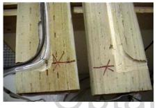
Here's how you will want to mark where you will run your 3/8" Cove bit in your router; in pieces A, mark a turnout where the lines will drop out of the wood at about 5" before the very end where the guy will be hanging from. Then mark all the way down the center and out the end of each. Above is a shot of the bottom of pieces C.
