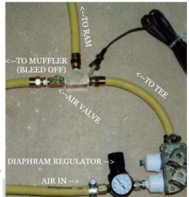
Once released the air travels to a three way connector that will split the air to the air cylinder as well as out to a muffler fitted at the end of about 5 feet of line. You can see there is an air valve to the muffler line because we will be dialing in the exact amount of bleed that allows our pneumatic prop to reset.
