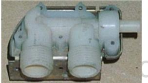
Of course you will need a water valve from a washing machine and not just any valve will hold the air back and reseat itself under the rather high pressure I would need for an air cannon. I wound up testing many, many different valves to see which work and which don't.
