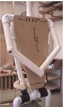
Three slots will need to be cut out as you can see for the wood to slip over the PVC pipe and the plunger from the air ram.
