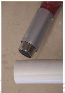
To round the end of the upper section I used a wine glass, as it had a rounded bottom inside and I need to use that as a mold for the plastic. The heat gun brought the PVC up to a soft, pliable point in just a couple of minutes and I simply pressed the end to the bottom of the glass and held it there until the plastic cooled.
