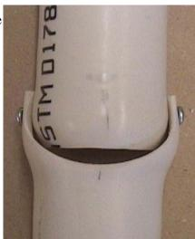
the top piece to move freely inside the joint. So how did we round the one and bell the other? It wasn't that hard.
