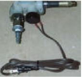
And here is how it will look when completed. The top of this photo got cut off, but you can see that 3/8" air hose slips perfectly over the outlet nipple for feeding the air to your prop. And that's it!
