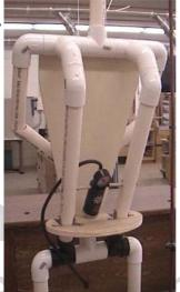
plunger slot dead center and the wood down almost as low as you can get it and still clear the lever assembly underneath. As you can see I merely held this in place with two 1" X 1" L brackets.
