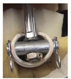
The massive plunger on this air cylinder that was mentioned at the start of this how-to, is 3/8" in diameter! So out of the lever comes the old steel rod, the PVC lever is drilled out with huge 5/8" holes and a section of 1/2" electrical conduit is drilled and fitted for the ram's plunger and the hitch pins.
