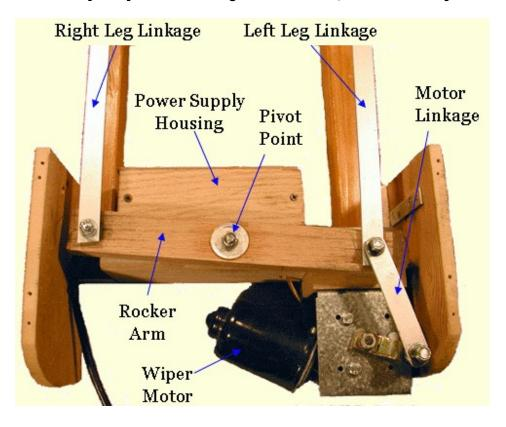
The leg linkages connect to the rocker arm using 1/4" bolts, t-nuts, washers and nylon insert lock nuts. The bolt and t-nut is shown below.
