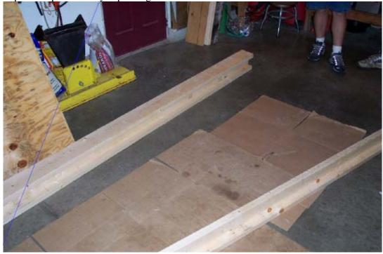
This photo shows our first idea for supporting the bridge. We figured that by creating our own I-beams, we could support the bridge across a 24 foot span. We were wrong. Our major problems occurred at where the two pieces of the bridge met in the middle. There just had to be a better way!
