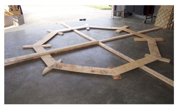
You can see the first layer on supports, and an arm that the router will mount to.
