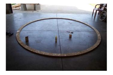
The process of assembling these rings is pretty easy. If you don't have to make these movable, you can just make each ring into two haves, and assemble the halves around the bridge. We needed to move these rings quite a distance in small vehicles, so these come apart into 4 sections.
