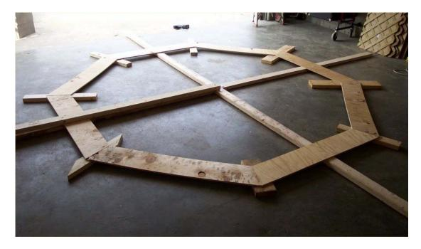
We tried building a big floor jig, that would simply allow us to take the router around the inside and outside edge of the ring, cutting the circle. This didn't work too well, but I will explain more later.
