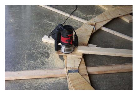
Here is a shot during cutting. This method would have worked great if the router bit was 1/2" longer! It was just short, and wouldn't cut both layers at once. We made the mistake of trying to flip the ring over, which didn't work. We ended up with a ring that had two cuts that did not line up.
