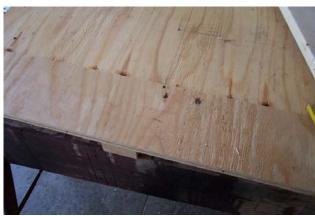
A board is mounted on the jig with two screws, and sometimes one in the middle. This prevents the board from moving around while we cut it.
