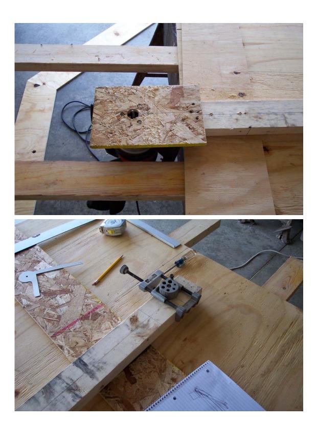
Making the pivot hole tight and straight was very important. We didn't want to develop any stray during the process of cutting everything.
