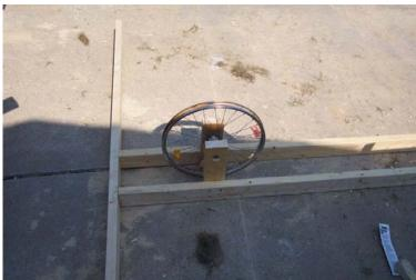
The base is made out of 3 of these things, one for each ring. Some 2x4's and bicycle rings are all that are needed.
