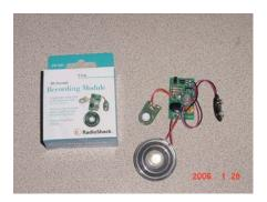
Here are pictures of the <u>Radio Shack "20-</u> <u>second recording module" (Part#276-1323</u> <u>\$10.49)</u> before and after hacking it to work with the PROP1 board and external speakers.
