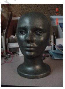
Worked out a few bugs in the PROP1/BS1 stamp code and now have that working pretty well. The PIR gets tripped, the PROP1 delays 15 seconds then turns the head around (via servo), lights the eyes up, and triggers the sound module. 20 seconds later the head turns back around and the eyes go out, and the PROP1 pauses for 40 seconds to ensure it can't be re-tripped right away.
