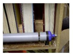
I positioned the remaining "haunted" books in amongst books that still had their contents and then marked on the PVC where I intended to make my remaining cuts. I rotated the PVC between cuts to create the cam so the books will move in and out at different intervals.
