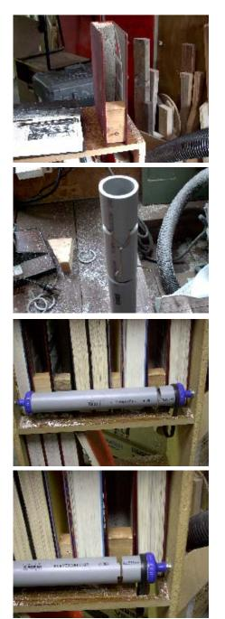
I wanted to test my idea by animating one book first so I started out by cutting almost all the way through a piece of PVC with my miter saw but stopped with about an inch left attached. I then used a piece of coat hanger to manufacture a push rod and soldered it so it wouldn't catch as the cam pivoted.
