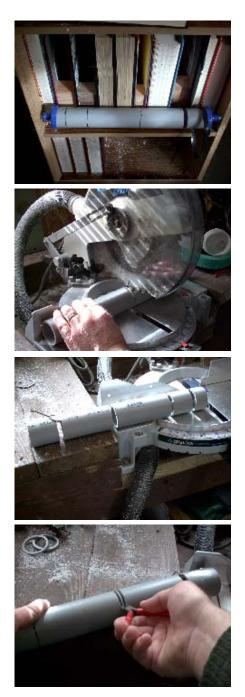
I manufactured push rods to match the others, attached them to the PVC and soldered them. I then attached them to the eye screws on the books and mounted the whole works back in the bookshelf. I had an old blender motor that I was able to mount underneath and attach the belt to.
