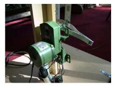
The vertical bars and center support are to be painted flat black to disappear into the darkness. The motor is a VERY heavy duty 6 RPM surplus motor I found online [picture at right] with a counter spring to help it come back up, the tried and true Dayton would probably work very nicely since the weight of the whole framework is basically all on the two center bolts supporting the vertical members.
