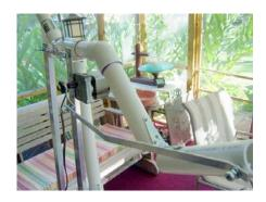
The arm crank mechanism is rather simple [pictures at right] but I had to rethink the way I did it again. I made a waving Bucky last year and the arm mechanism worked great using the elbow joint as a hinge. I got it to work on Harry but unfortunately, it was prone to locking up so I opted for PVC and a strap hinge. I thought about linking the arm to the leaning motor but opted not to; I wanted the arm having independent hitching movement for a more lifelike (or deathlike) look.
