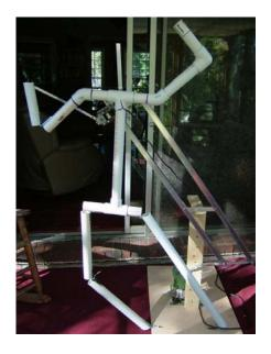
So here's how I did it and the mistakes I made and things I learned... First of all, the key to the 'natural' movement of the body is that the center bars that connect the large vertical parallel bars are always horizontal, therefore the body could be attached to that and it wouldn't lean over as the verticals tilted side to side [as shown at right and below. Text continues below.]
