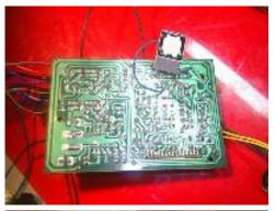
On one side of the board are the wires that work the Santa motors and the speaker. I remove then here to show the blue and green wires. I connected them to a 9 volt relay.
