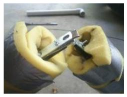
Close up of the knees. they are just hinges. I placed a piece of metal over the top stop the leg from bending one way.
