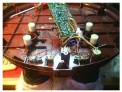
Here is the bottom of the dancing Santa. For the hangman hack I used the chest and arms, the circuit board, and the rods for the legs.
