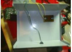
I bought a project box at radio shack to hold the components. Here you can see the start button and the motion sensor installed.
