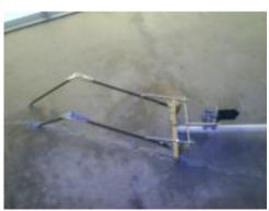
Here is the Kicking rig I made for the hangman. In the picture you see that at first I wanted to use springs to pull the legs up. It worked great in my first tests but later after the prop was dressed they did not have the power needed to lift with the extra weight.
