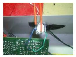
Wires were soldered to the relay to power the wiper motor that will run the hangman. The wiper motor is powder by a 15V 1 amp power supply. One wire from the power supply goes to the wiper motor, the other goes to the relay. The other wire on the relay will go to the other wire on the wiper motor.
