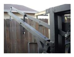
Link arms are attached to the bell cranks which Bluckies are mounted on. End result is that the Bluckies "swing" back and forth.
