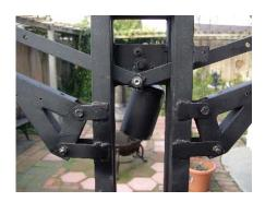
Limbs in place and link rods attached to crank. Rotation of the crank produces a back and forth movement.
