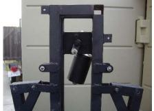
The crank arm of the wiper motor can be seen here.
