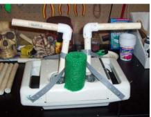
Now add the 8" pipes and the 45 degree and/or 60 degree fittings as shown
