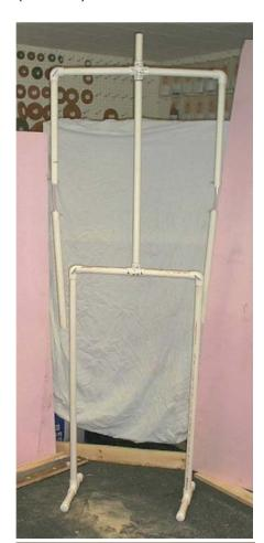
If you need more pivot points, just cut slots in the 90 degree pieces and screw them in as well. On a final note paint everything black or white depending on what you are creating and spray a little silicon lubricant on the moving joints for a smoother operation. Pic #11 shows the finished frame.
