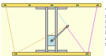
The drawing at left shows the routing of the three pieces of fishing line. After it passes through the front screw eyes, leave enough hanging for attachment of the skeletons as shown below.
