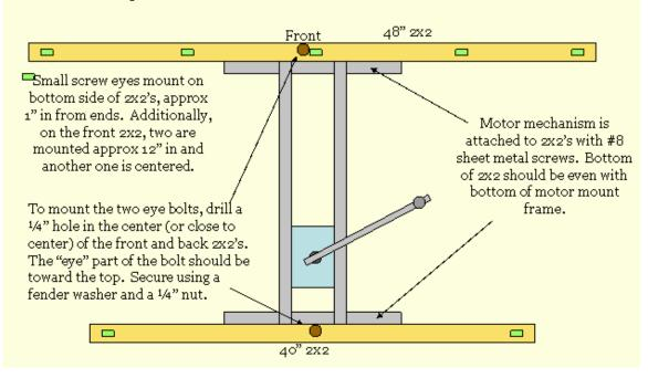
Attach the front and rear 2x2 boards to the motor mechanism as shown above.
