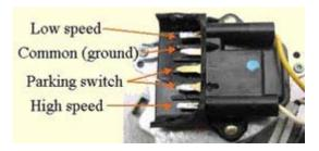
Before mounting the dancing skeleton rig to the ceiling, you'll need to wire up the motor. I recommend wiring it for low speed operation by attaching wires to the "low speed" and "common" terminals as shown at right. Note that part of the plastic housing has been cut away for easier access to the terminals. Soldering is the most reliable method of wire connection. For more info, see my <u>Wiper Motor Pages.</u>
