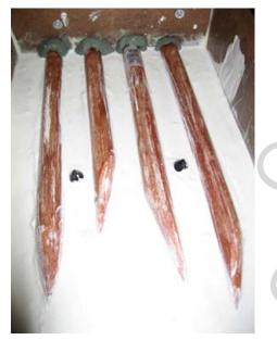
Believe it or not, this was the toughest part. I recently figured out how to make latex molds so I figured this would be easy. I carved four spikes from 1" wooden dowels and made a latex mold. I then got some 2-part 8lbs polyurethane flexible foam, mixed and poured.
