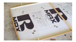
I then numbered the skulls and placed them on the foam board in the arrangement I wanted. I marked the placement of the eye sockets and drilled out 1.5" holes. I put a numbers by the holes so that I could match the skulls to the hole pairs later on.
