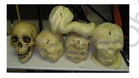
Working with two-part polyurethane foam takes practice. The key is in the mixing. I used a bend coat hanger stuck in my power drill and mixed the components in a clear plastic cup. By the way, make very sure you don't have any sharp edges on your mixing blade if you do this. I always tested out the mixer in the cup before I poured anything in it and
