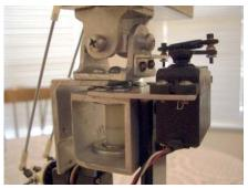
Tilt and nod are done with the use of a "V tail mixer" available at most hobby shops made by DuBro who also makes a great assortment of linkages and small parts used on radio controlled (R/C) model airplanes.
