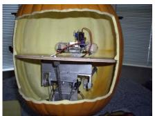
With lots of room left over, I fabricated some 2 axis eyes. Again, using cut up scraps of various aluminum shapes. Since there was almost no force required to move the eyes, micro servos were used. I'll do a how-to on the eyes at a later date, for now, here's a couple of pics.
