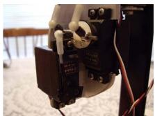
You can see here the upper attachment of the 2 link rods that control tilt and nod movements as well as the pan servo mount.
