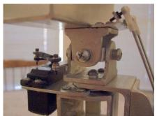
The pan servo with linkage to the base of the U joint.
