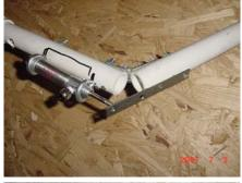
The Bimba cylinder used only has a 1" movement (which is all I needed to move the arm from a 90-degree position, to a slightly dropped position when Private Waltrip lights the cannon). The elbow is a simple hinge screwed into the PVC; the cylinder providing the motion is mounted behind the arm and held in place by two eye bolts that I found that just happened to be the right size to hold the cylinder in place.
