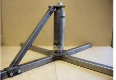
Rear braces are added to keep the spindle assembly securely in position.
