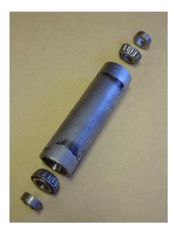
This photo shows the rotating portion of this spindle. In the lower left corner you can see the bearing's outer race is installed in the outer case. You can also see round plug welds roughly one inch from each end of the outer case. Holes were drilled through the case, and when the outer race retainer stops were in the proper position, they were welded in place through these holes.
