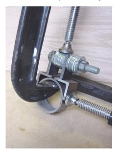
I have been making my own clevis mount brackets all along. Shop made mounts can be any shape or size completely customized per prop, per application. The photo above shows the lift cylinder clevis mount ready for welding.
