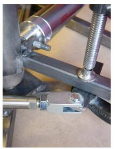
With the cylinders and their mounting brackets connected, it's easy to clamp the brackets to linkage components for test fitting. Clamp each end securely and manually move the part. If needed, reposition the mounting bracket and test again. Once satisfied with the joint's range of motion and acceptable clearance(s) it's safe to tack the mounting brackets in place. Remove the clamps and test the motion again.
