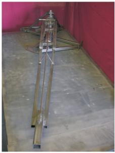
As previously mentioned, the lift arm for this machine will be fairly long. Any combination of substantial weight and sudden changes in motion would cause a long, thin arm member to flex. To eliminate this flex without using a heavy walled single tube (which would add even more weight at the end of the arm) I decided to break the arm into two segments.
