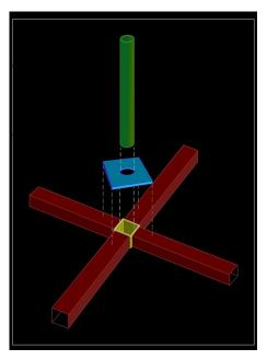
This drawing shows the individual components of the spindle base. The yellow colored square tubing in the center of the
