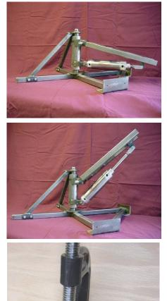
These photos show the Bellicose machine with lift cylinder retracted, then extended.
