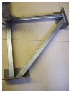
Directly opposite the rear brace assembly, the remaining two legs of the spindle base are joined with a cross brace.
