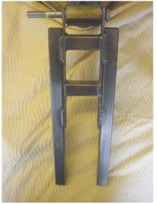
This is the base section of the lift arm. This mounts to the pivot joint attached to the spindle.
