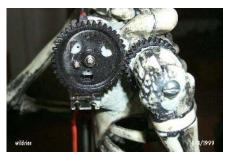
When you choose a <u>servo</u>, there are two numbers that you want to look at. The Torque and the Speed. The shoulder requires a 60 to 100 oz/in servo, but a slower speed servo in this case is better. The servo will only move about 180 degrees. With the gears that I chose, the small gear will turn about 3/4 of a turn, giving the arm a range of over the head to behind the back which is about what a human arm will do. Since
