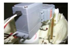
Here are the servos mounted inside the skull. The jaw servo is connected to the jaw lever (piano wire) with a piece of square brass tube with a hole drilled in either end. When I took this picture, I had a spacer between the control horn and the brass link, but I later removed it to make things align better.
