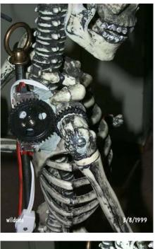
The side view shows the gears used to move the shoulder. The small gear is attached directly to the arm. It is driven by the larger gear which is attached to the servo. The servo is connected to the skeleton with epoxy.
