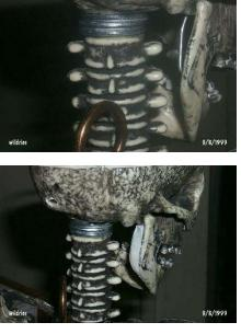
When the servos turn the head and the jaw opens and closes, the jaw hits the collar bone. To reduce this problem, I added metal washers on the neck to lift the skull up a bit higher so that when the jaw opens, it will clear the collar bone. Three washers are not quite enough, but any more and the neck does not protrude into the skull enough for control.
