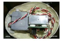
Here you can see the routing of the servo wires to the PC board and the putty holding the PC board to the side of the neck servo.
