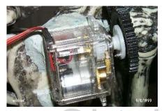
Next I took a <u>CIRRUS CS-60BB</u> servo I purchased from <u>Sheldon's Hobby</u> for \$24.99 and replacing the short center screw with a longer one from the servo parts pack, I attached a T40 gear (from the same 5 pack I got above) to the servo horn (the white piece). I drilled a small hole for an additional screw to tie the servo horn and the gear together.
