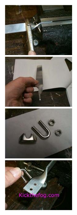
Take your 12" cut piece of flat aluminum and place about 1 1/4" of it in a vise. Using a pair of vise grip pliers, grip the aluminum about 1 1/2" away from the vise. Bend the Aluminum 90 degrees. I was shocked to learn how easy it was to bend using a vise and vise grips. Without these, I don't know how you'd bend it
