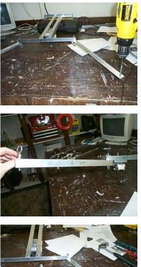
Here you can see in this <u>bottom view</u> of my frame that we have both arms secured to the frame using eyebolts. Now we must drill holes in the ends of the arms. Do this also with your 1/4" drill bit and center the hole on the end like you just did to mount the arms to the frame.
