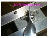
In the picture, here, I have them tightened pretty good (Don't over tighten or you'll break the u-bolt!) and you can see the snug fit between shaft and ubolt.
