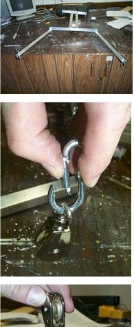
That's it...your frame it built! This gives you a pretty good look as to which eyebolts are pointing up and down. The 4 eyebolts on the frame face up. The 3 eye bolts, 1 on each arm end and the 1 in the center of the rear frame, face down.
