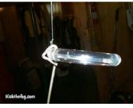
As you can see, I secured the ring by bending the end of the arm around the ring.
