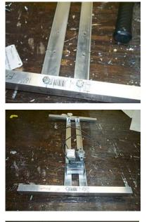
Drill the 4 holes you just marked with a 5/32 inch drill bit and enlarge if necessary. I had to enlarge mine with a 3/16 drill bit because I must have moved the paper a bit while marking (they didn't quite line up even with being able to move the aluminum)
