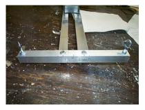
Turn your frame around. Drill and mount 2 more eyebolts the exact same way you did the others at the ends of the rear frame just like you did for the front. These will be pointing upward and will serve as the mount points to the ceiling.
