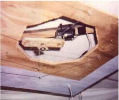
The motor's mounting beam is made of plywood, and is screwed to the large piece of plywood on plywood legs to hold it up so the crank is at the same level as the large piece of plywood.
