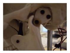
The first thing needed was a solid, smooth operating jaw hinge. After a little work with a Dremel tool I mounted a small piece of aluminum to the skull and used a 4/40 bolt through a nylon bushing into the jaw as the pivot. You can also see the rod attachment to the jaw in the pic below.
