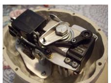
In this pic you can see the pan and nod servos. The center shaft remains stationary while the skull pivots around it on bearings in the pivot block. The nod movement is done by the servo moving the mounting plate up and down.
