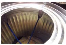
8. Put the bungee and canvas into the top of the can and secure the bungee hooks to the four eye bolts with Duct Tape so that they will not come loose when firing.
