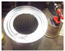
4. Drill four 1/4in holes equidistant around the large hole in the bottom of the can using one of the large washers as a guide to how close to the edge you can come. Then place one nut and lock washer on the eye bolts. The eye will be on the inside of the can for the bungee straps to attach to. Insert them and then top them with one large washer, one lock washer, and one nut and tighten down. The large washer is to prevent the bolt from pulling through the metal when the bungee are pulled back.
