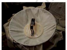
10. Cut off any excess canvas and attach a handle. I used a fog machine bracket and secured it with drywall screws. Then I coated the canvas with straight latex for good measure to make it more airtight.
