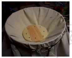
9. Now turn the can right side up and situate your canvas diaphragm across the opening. The wood center should just pull the bungee tight without actually stretching them. The can top has basically two ridges on it. Using the 48in bungee secure the canvas below the second ridge.
