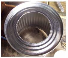
1. Using the same proportions as a real AirZooka cut a hole in the bottom of your garbage can using a jig saw. It goes without saying - OK I'll say it. Use all safety equipment (IE gloves, protective eyewear, etc). Multiply the diameter of the bottom of your can by 0.2 and this will approximate the rim thickness.
