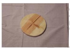
3. Once sandwiched together use drywall screws to secure it together. Flip it and do it to the other side offsetting the screws. Always pre-drill all holes for screws to avoid sad mishaps
