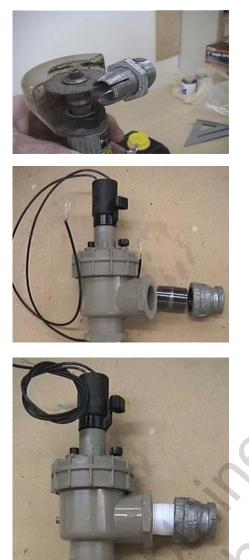
It's true, the sprinkler valve has been used for some months now for air cannons, but they produce a hollow, almost "honking" sound which is loud, but not very desirable. So once I built my prototype I hoped I could come up with a modifier to this report.
