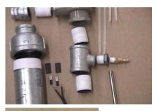
Next, let's get our air cylinder together. Be sure to use teflon plumber's tape on all the threads of the fittings and make sure all of your connections are very
