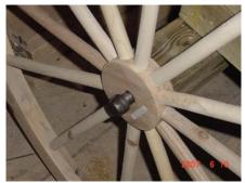
1/2" pipe "end caps" screw onto the end of the axle to hold the wheel on (which will have washers added later). We decided on 36" for the length of the axle based on the size and scale of our cannon.
