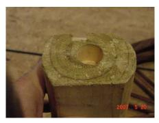
First we mounted the two wheels on a 4x4 axle. The wheels came with wood dowel inserts which we inserted into drilled out holes in the ends of the 4x4. After testing this we decided a sturdier axle was needed.
