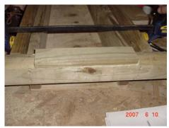
We also had to flatten the front lip of the axle so we the side mounts that hold the barrel would sit evenly. These are pics of the notched front end.
