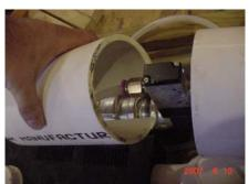
The valve attached to the QEV has a manual firing switch, which allowed us to test it before we hook up all the controlling electronics.
