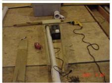
By test fitting the pipe and fogger, we decided on a width of 14" nearest the barrel, tapering off to 11" at the base; the undercarriage is 4' long.
