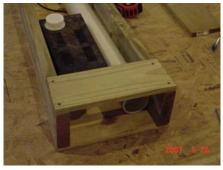
Next we started assembling the undercarriage. This had to be wide and deep enough to hide the fog machine and a pair of 2" wide steel pipe inside it, yet still look as realistic as possible.
