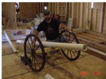
We fastened the undercarriage to the axle using 4 4" galvanized deck screws.
