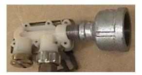
In this shot you can see where I have taken a  $2" \ge 1/2"$  threaded fitting and inserted one end into a T fitting to use as a handle as I prepare to make a thread tap. Then the end remaining I used a die grinder to slot the sides in 4 places, about 1/2" up.
