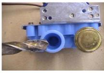
N-51 valve for a cannon. You will need to drill this back past the inlet port inside the valve that is coming up from the cylinder. On the same valve I show doing the same thing to the inlet port. Note that this is the closest inlet port to the exhaust port as
