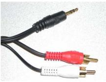
This cable plugs into a CD player and sends the sound to two RCA jacks. We only need one of them to plug into the lightning machine.
