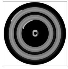
Using the epoxy product we used earlier, attach the metal rings securely onto the top of the black PVC end-cap. Make sure the rings are centered around the motor shaft as evenly as possible. After the epoxy sets you can use a dremel tool to gently remove any excess adhesive that may have found its way onto the metal surface.
