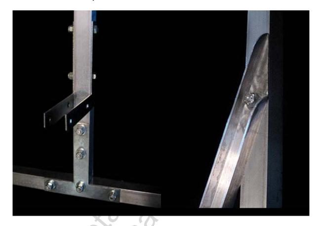
Repeat this process to create the second leg. The second leg must mirror the first with the angled channel and "L" brackets facing the opposite direction of their counterparts from the first leg.
