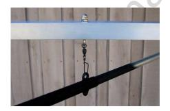
The mechanical lever is made from a 72 inch length of  $5/8 \, x$  .093 round aluminum tube. You may find that you need a lever of a different length depending on the width of the window or display area in which you intend your prop to float. For the 32 inch opening of my window display this length works quite well.
