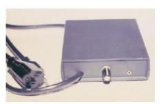
As the name implies, this is a no-frills controller. Input is direct audio via a 1/8" audio jack. A sensitivity control is provided.
