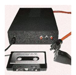
Unlike most other lightning controllers that take a thunderclap sound and turn it into light, this unit includes the thunderclap sound on a digital chip.
