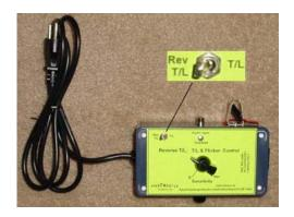
It consists of a single-channel color organ, with a sensitivity control. It handles 600 watts. Input is via direct plug-in connection, isolating the effects from ambient noise.
