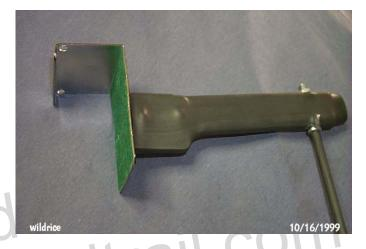
I then cut it off, drilled a hole through it, and inserted a length of 1/4 inch threaded rod. I used a wing nut on the bottom of the hanger because of the way it was made. Finally I covered it with heat shrink tubing.
