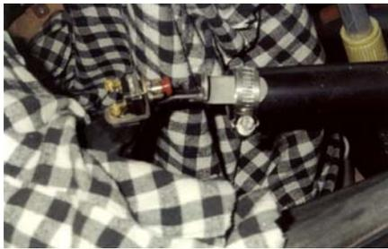
This is a normally open momentary button I picked up at OSH. I screwed it to the bracket that my screen door closer air cylinder attaches to his arm.
