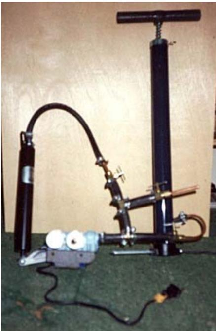
This works perfectly, but use plenty of screws & fender washers, so the pressure of plugging in the air cord doesn't rip the screw heads out of the plastic.
