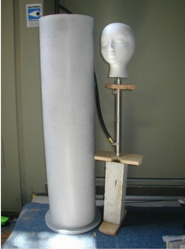
Pneumatic cylinder and blocking inserts in the column, so the top of the styrofoam head is flush with the lid.
