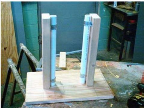
I centered the 2X4's, fitted the skeleton pipe so it slid up and down smooth and screwed them to the plywood.
