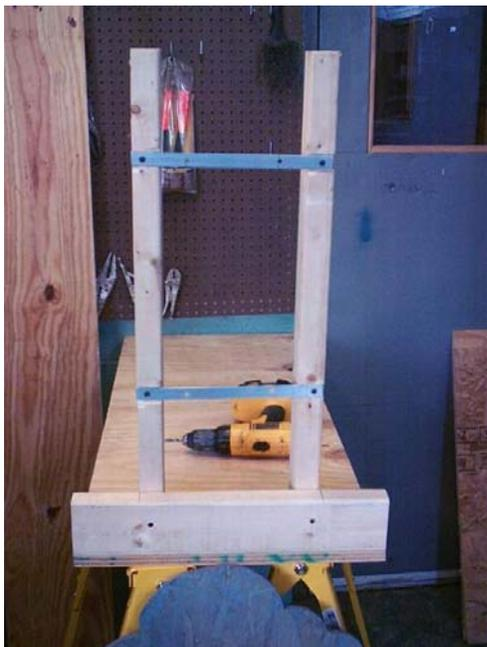
I built a frame to hold tombstone, I want mine attached, all one piece. Notice the metal bars have holes in them. I placed the cut out board on frame and drilled holes.
